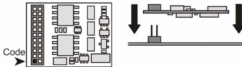
To install the decoder simply remove the dummy socket in your locomotive and install the decoder plug. Ensure Pin 1 of the decoder is aligned to Pin 1 of the locomotive. When installing the plug ensure that the pins are not bent or broken
